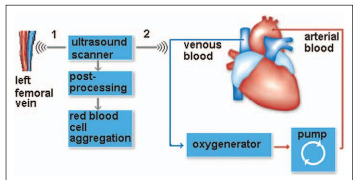
**Figure 1.** Cardiopulmonary bypass setup and radiofrequency ultrasound acquisition in the swine's left femoral vein (1) and the pump circuit (2), with a high-frequency ultrasound scanner.
